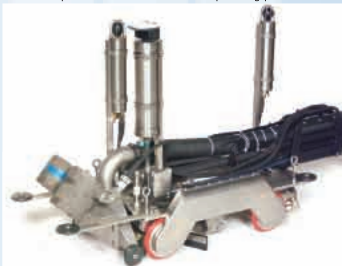
For cleaning and inspection, the OTIS robot is equipped with a vacuum system
