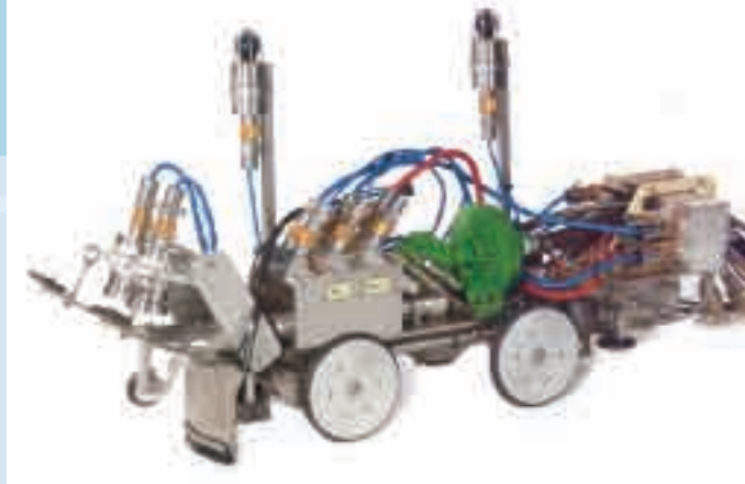
The OTIS robot configured for inspection service without optional cleaning
